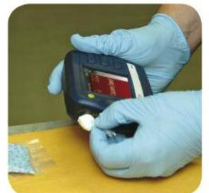
Analyze through sealed packaging for most samples.
